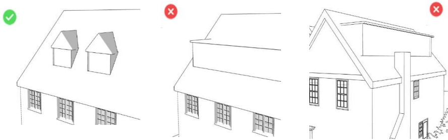
Figure 7 - sketch diagram showing dormers that are an appropriate size and position, and examples of proposals which would not be accepted.
